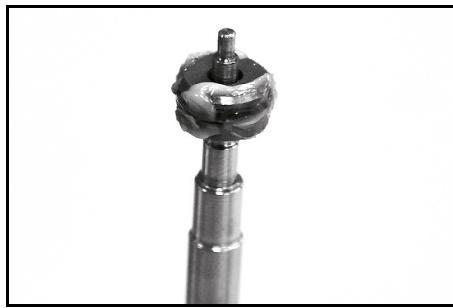
6. Grease the seat with silicone grease (part number 6.288-044.0).
