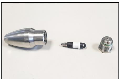
4. Press out the seat with the special tool (part number 6.025-233.0).
