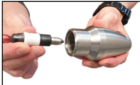
9. Grease the thread of the cap with grease (part number 6.288-079.0).
