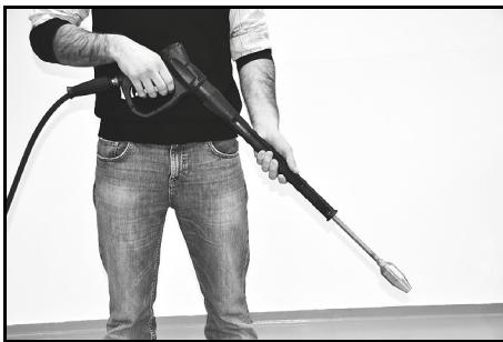
2. Start the cleaning work with a nozzle clearance of 20 to 30 cm. Determine the best nozzle clearance by slowly approaching the cleaning object.
